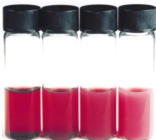
Fig. 11 Photograph of Au@SiO 2 colloids (15 nm core diameter and 83 nm shell thickness) as a function of the mixed toluene–ethanol refractive index. The refractive index varies from 1.36 for the sample on the right to 1.456 for the far left sample. 85 Reprinted from Langmuir , 1996, 12 , 4329, copyright 1996, American Chemical Society.
