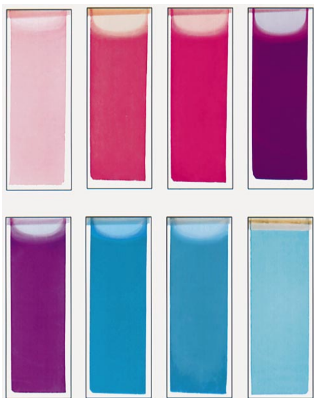
Fig. 15 Photographs of dense Au@SiO 2 films with 15 nm diameter core gold particles, and different shell thicknesses. The top left film is a sputter coated gold film. The next two bluish films are formed from gold sols which have sodium citrate (0.5 nm) and sodium mercaptopropionate (1.0 nm) shells, the other films utilise gold colloids with silica shells having thicknesses: 1.5 nm, 2.9 nm, 4.6 nm, 12.2 nm and 17.5 nm. The shell thickness controls the dipole coupling between particles and hence the colour of the film. The homogeneous particle size ensures homogeneous film colour. For shells greater than about 15 nm in thickness, the particles are almost completely isolated, and the transmitted colour is similar to that of the colloid. As the shell thickness is reduced, the colour shifts from red to crimson to purple and finally for 0.5–1 nm thick shells to a blue colour similar to that found for conventional evaporated gold films. The reflected colour also changes gradually from a green tinge through to a metallic gold colour as the coupling increases.
